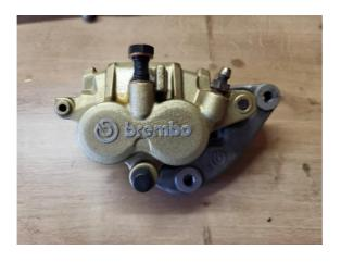
o Original *Brembo* front caliper (1996–2003).
